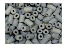
Guardian-CR is a hollow CoMo cylinder with mild activity designed for use as top bed grading in a variety of hydroprocessing unit applications. In addition to excellent physical integrity, Guardian-CR provides high void space for particulate trapping. These rings, along with Guardian-CT trilobes, are typically loaded above the main bed catalyst and aid in providing even flow distribution.
