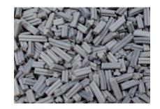
Guardian-CT is a CoMo Trilobe designed for use as bed grading in a variety of hydroprocessing unit applications. This shaped extrudate, typically loaded below other inert and active gradings such as Eurecat's Guardian-CR CoMo Rings, provides even flow distribution and pressure drop control along with moderate hydrogenation activity ahead of the main bed high activity HDS/HDN catalysts. Guardian-CT also offers excellent physical integrity.
