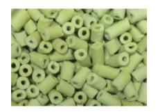
Guardian-NR is a hollow NiMo cylinder with mild activity designed for use as top bed grading in a variety of hydroprocessing unit applications. In addition to excellent physical integrity, Guardian-NR provides high void space for particulate trapping. These rings, along with Guardian-NT trilobes, are typically loaded above the main bed catalyst and aid in providing even flow distribution.
