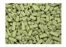
Guardian-NT is a NiMo Trilobe designed for use as bed grading in a variety of hydroprocessing unit applications. This shaped extrudate, typically loaded below other inert and active gradings such as Eurecat's Guardian-NR NiMo Rings, provides even flow distribution and pressure drop control along with moderate hydrogenation activity ahead of the main bed high activity HDS/HDN catalysts. Guardian-NT also offers excellent physical integrity.
